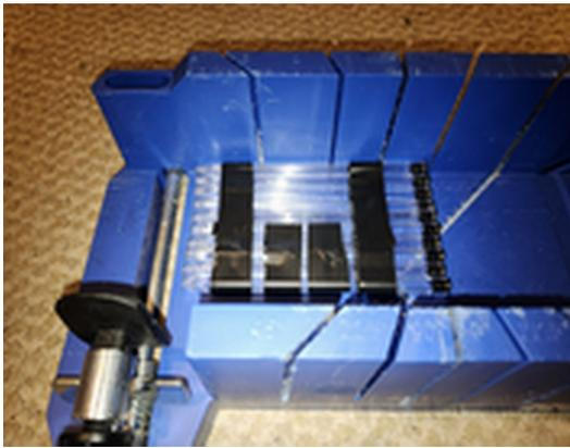
When all the spacers are cut, it is time to start assembling your ladder line. Cut off two fifty-foot sections of your wire. Set the wire aside for now.
