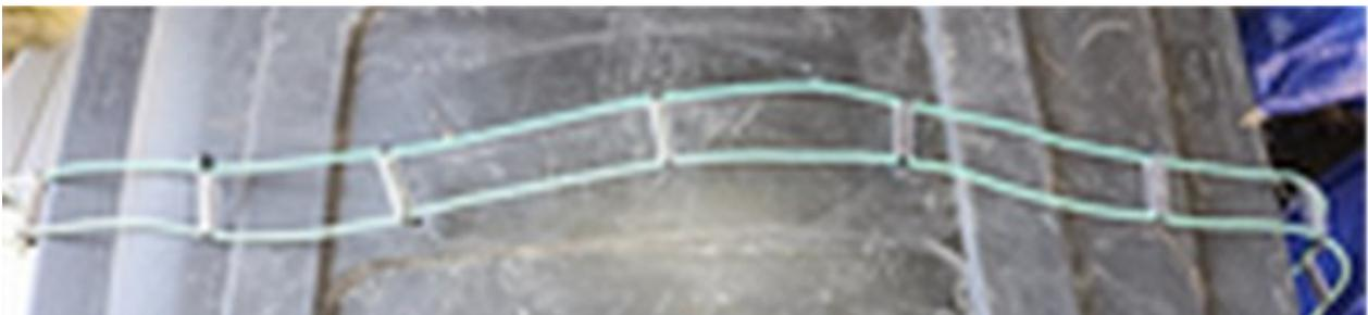
I made two sections of ladder line. They were both ten feet long and are going to be used as the matching section for the Extended Double Zepp antennas I am going to experiment with.
