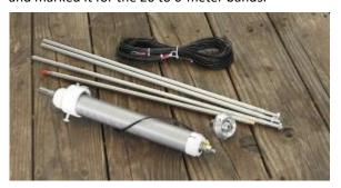
However, I have changed the radials from 12 to 20-gauge wire so the carry bag is lighter, and they are easier to set up. I also went with three sets of four 16.5' radials attached to a clip that is attached to the tripod legs.
