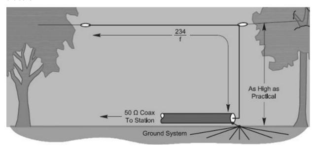
The antenna has a 3:1 or higher SWR on most bands. The only bands that are so bad that the internal auto tuner on my Kenwood TS-590s won't handle are the 160 meter and the upper portion of the 75-meter bands. This is why I am considering a balun of some sort for this antenna. In the meantime, I am using an external manual antenna tuner to use these two bands.
